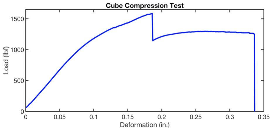
Figure 2: Load versus deformation of the polycarbonate cube.
