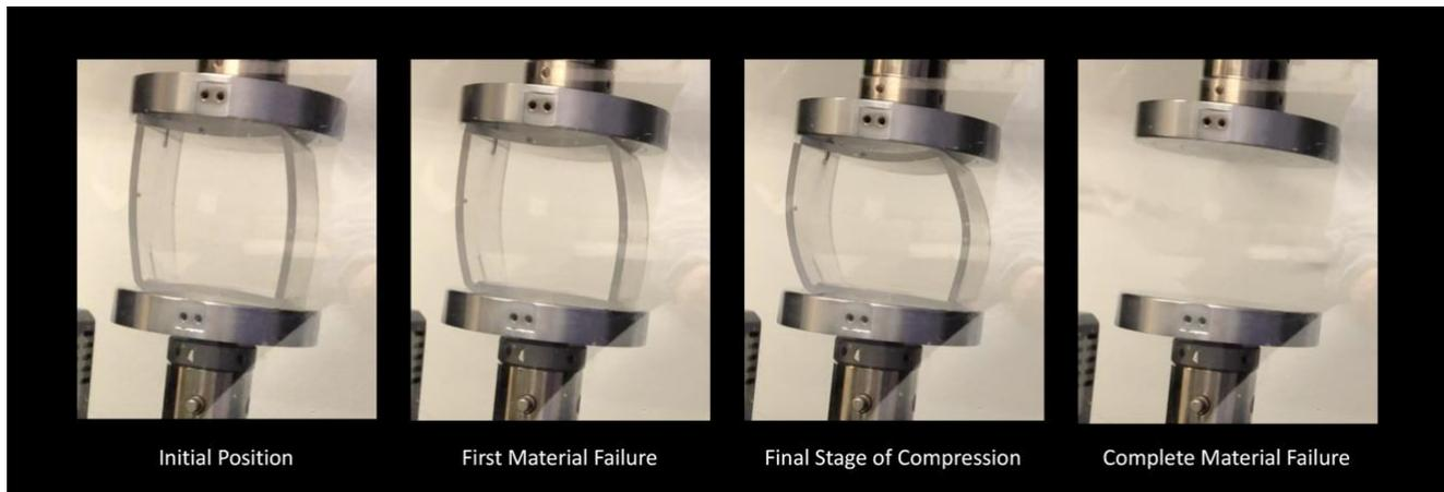
*Figure 1: Setup for cube compression test and different stages of compression until final failure.*
